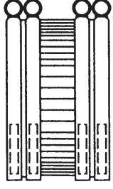
Sizes 5" thru 10" Tighten inside clamps first, then outside clamps.
